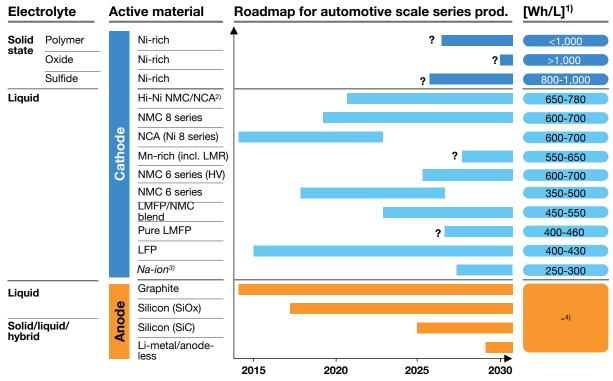
1) Target values for supplier of pouch or prismatic cell; 2) Ni 9 series; 3) Not only cathode chemistry per se but listed for simplification; 4) Primarily driven by cathode chemistry
