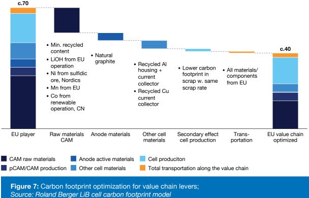
**Secondary effects:** The carbon footprint of scrapped materials is lowered if they came from  $low-CO_2$  sources. The footprint of scrap can therefore be reduced (by around 2 kg  $CO_2$ -eq/ kWh) even if the scrap rate stays the same.
