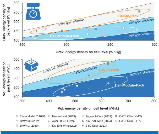
**Figure 17:** Gravimetric vs. volumetric energy densities on cell and pack level with respect to different pack architectures; *Source: PEM of RWTH Aachen University*
