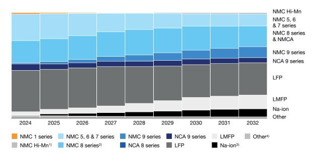
1) Incl. NMX similar to NMC271; 2) Incl. NMCA; 3) Na-ion share consists of the two cell chemistries nickel-based layered oxide and Prussian white; 4) Incl. LMO/LCO/...
