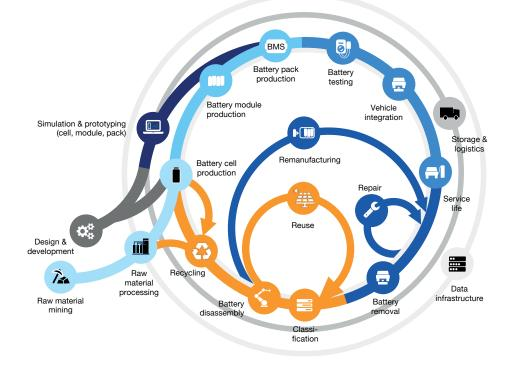
Figure 26: Battery lifecycle with different phases; Source: PEM of RWTH Aachen University
